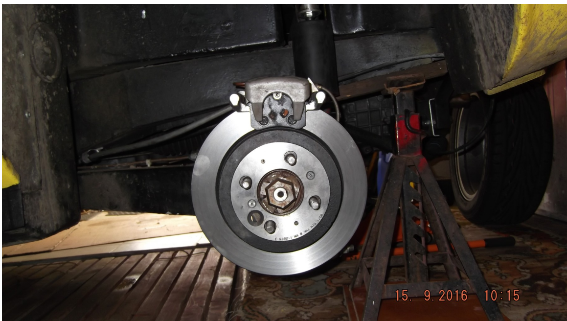
Fig 3 : Caliper finally in place
