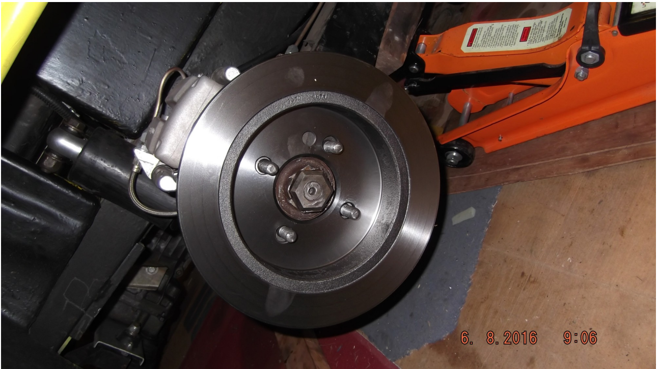
Fig 1. Trial Fitting of Mini Rear disc on Studs/hub
