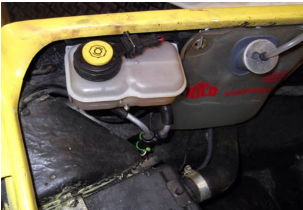
Fig 7 : Remote Reservoir with level switch
