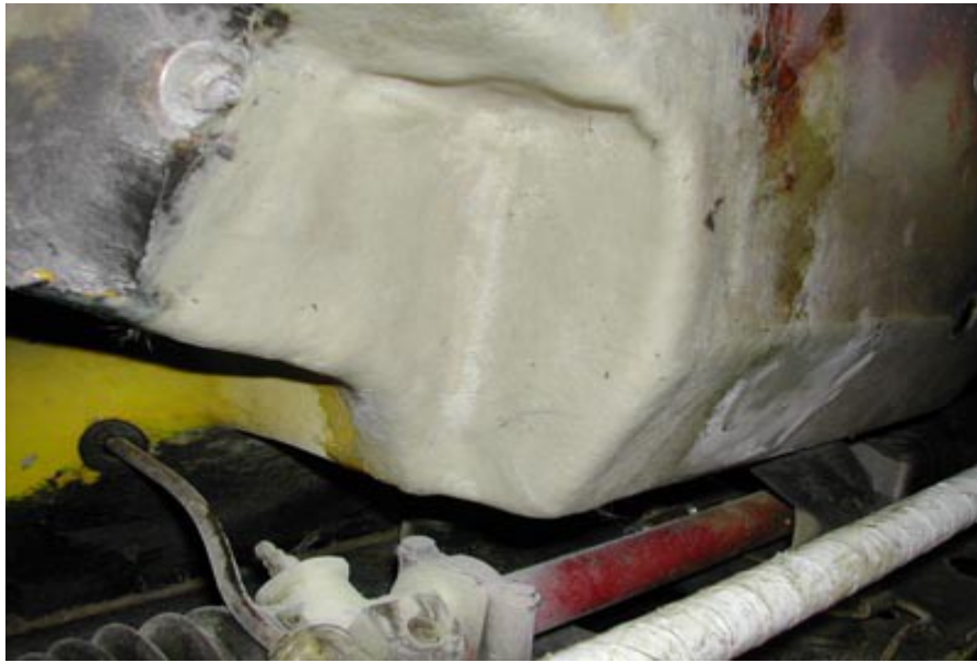
Fig 3 : Repair section in place (view underneath)
