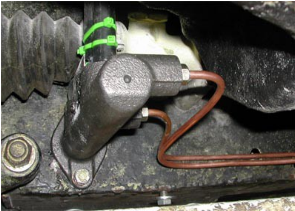
Fig. 6 : Modified undertray gives better access
