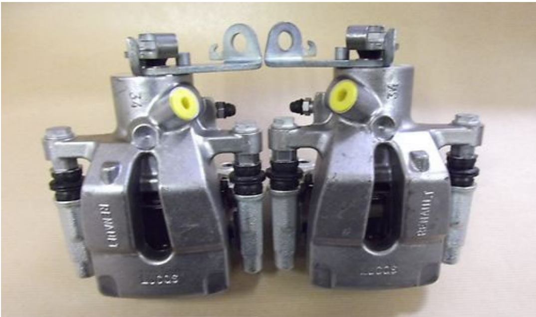
Renault Scenic 1999-2003 Rear Calipers Lucas Trailing Caliper. Solid 11mm Disc. 1x34mm piston
