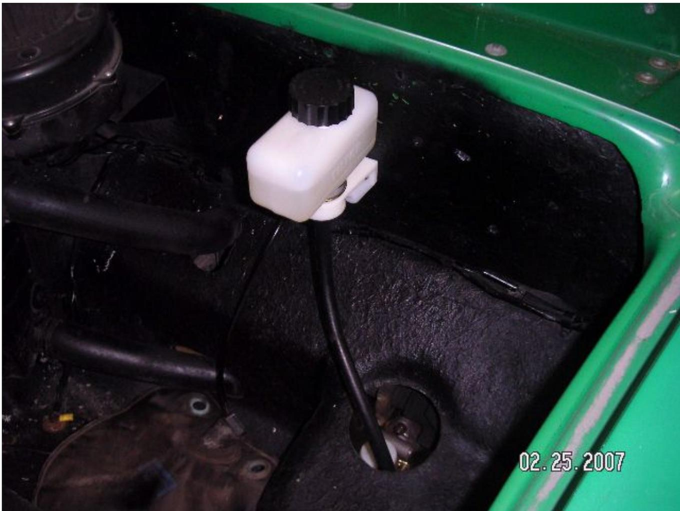
I installed the proportioning valve inline where the rear booster used to go. This made for nice uncomplicated lines at the master cylinder, and easy access in the engine compartment. I had originally considered installing the proportioning valve up front by the M/C but I like things simple, so I put it where it is. This picture below shows the proportioning valve installed. It's the small black box with the black knob just to the left of the header.
