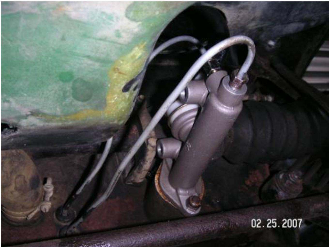
Note on the picture above, that the mounting holes on the Tilton are a perfect match for the Europa. The rod that links the pedal to the M/C needs to be moved from the original M/C to the Tilton... No big deal there, as it's a direct fit.
