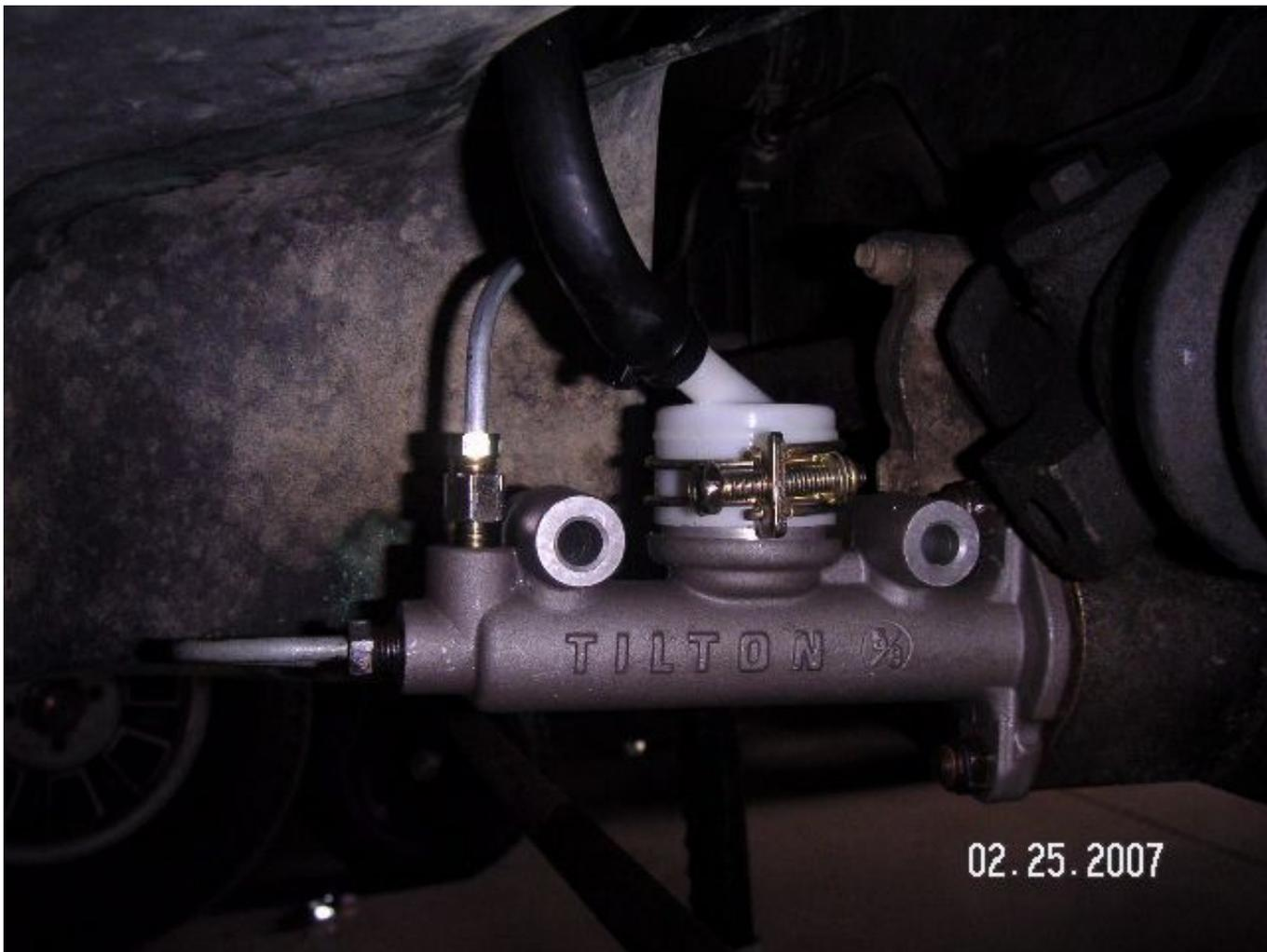
The Tilton kit comes with two reservoirs, plus a remote mounting kit. I chose to mount the large reservoir remotely because it fouled the steering rack when installed directly on the M/C. Picture below.
